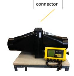
flanges. It is necessary that the pipe downstream from the counter is downward sloping all the way.
