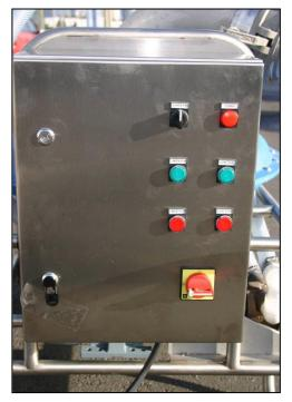
**1** Turn off the power at the main switch and open the door of the control cabinet. The door can not be opened unless the main switch is turned off.
