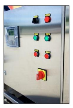
1 Turn off the power at the main switch and open the door of the control cabinet. The door can not be opened unless the main switch is turned off.
