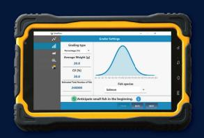
Settings of the grader can be adjusted to reach the optimal quantity of fish in each category.
